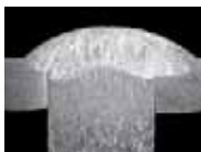
Cross-section of 360° Buttonless Weld
