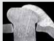
Cross-section of Traditional Bridge Weld
