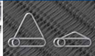
Patented Special Mesh Spirals A cost effective solution for adding lane dividers or flights
